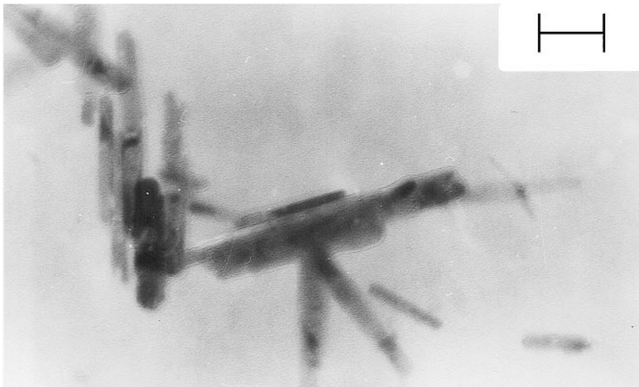
Figure 2. Scanning electron micrograph of \gamma\text{-Fe}_2\text{O}_3 particles. Bar length is 30 nm.
